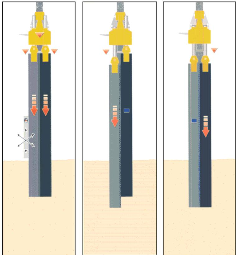
Once all piles in the group are advanced by the full stroke of all Push-Pull cylinders, the entire pressing device retracts, ready to repeat the cycle. This simple process is the same irrespective of the total number of Push-Pull cylinders.
